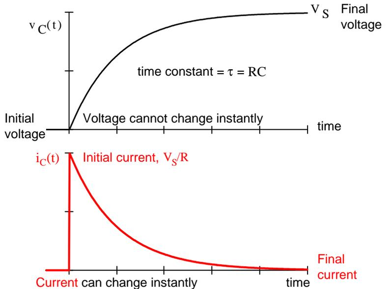
**Initial Condition** is typically found by finding the capacitor voltage just before time  $t = 0$ .
