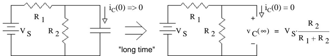
Replace the capacitor with an open and find the voltage across the open (just like finding  $v_{Th}$ ).
