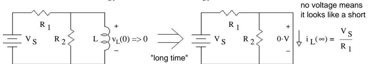
Replace the inductor with a short and find the voltage across the.
