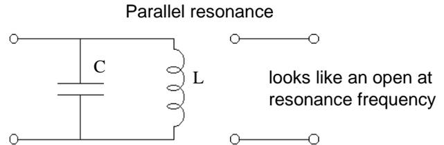
The resonance frequency is calculated the same way for either case:
