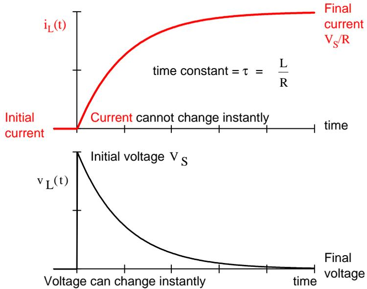
**Initial Condition** is typically found by finding the inductor current just before time  $t = 0$ .
