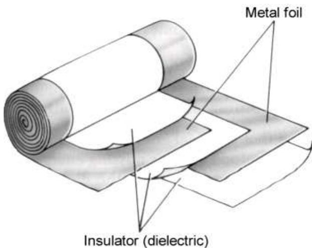
Capacitors are typically classified by the material used for insulation. The insulation determines some of the non-ideal characteristics. See Table 3.7 in text
