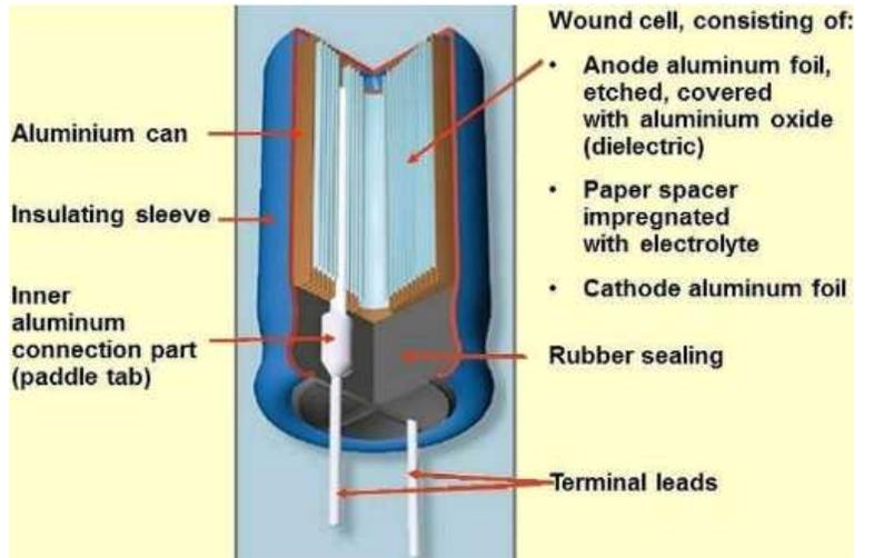
Almost all electrolytic capacitors are **polarized**. The negative terminal must always be negative with respect to the positive terminal, other wise it may be ruined.
