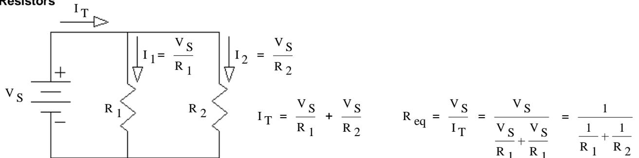
Resistors are in parallel if and only if the **same voltage** is across each resistor.
