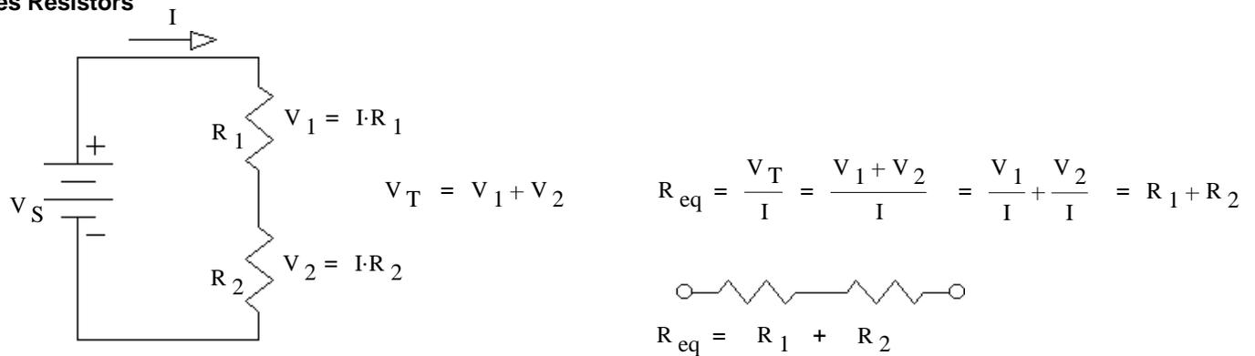
Resistors are in series if and only if exactly the **same current** flows through each resistor.
