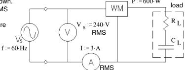
a) The value of the load resistor.  $R_{\tau} = ?$
