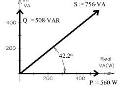
g) 93.6·μF capacitor in parallel with load
