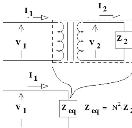
You can replace the entire transformer and load with ( $Z_{eq}$ ). This "impedance transformation" can be very handy.
