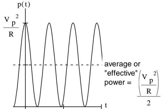
Couldn't we define an "effective" voltage that would allow us to use the same relationships for AC power as used for DC power?
