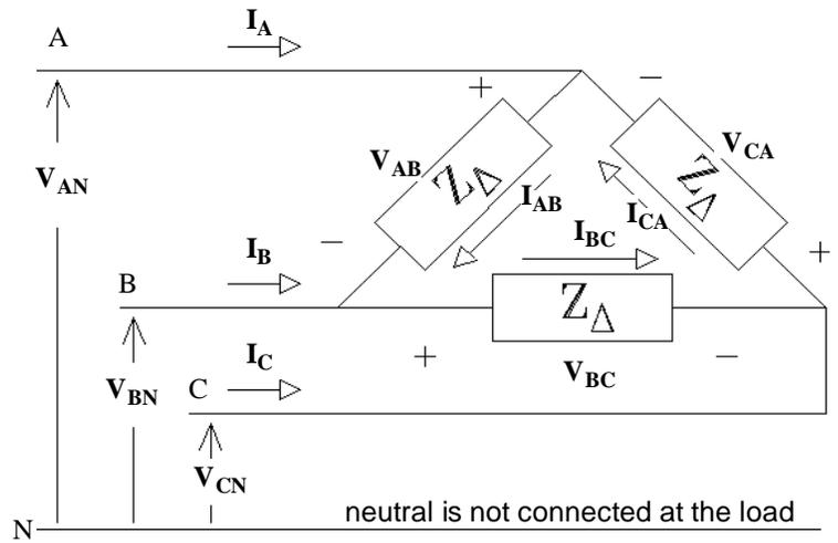
$|V_{AN}| = |V_{BN}| = |V_{CN}| = V_{LN} = \frac{V_{LL}}{\sqrt{3}}$
