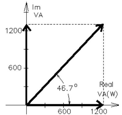
**Ex. 2** R & L together are the load. Find the real power P, the reactive power Q, the complex power S, the apparent power |S|, & the power factor pf. Draw phasor diagram for the power.
