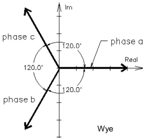
$$V_{LN} = \frac{V_{LL}}{\sqrt{3}}$$
