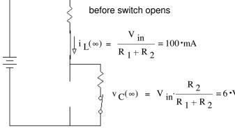
$\begin{cases} v_{C}(\infty) = V_{\text{in}} \cdot \frac{R_2}{R_1 + R_2} = 6 \cdot V \end{cases} = \frac{\frac{d}{dt} v_{C}(0)}{\frac{d}{dt} v_{C}(0)} = \frac{i_{C}(0)}{C} = \frac{-166.7 \cdot \text{mA}}{C} = -1.334 \cdot 10^{6} \cdot \frac{V}{\text{sec}}$
