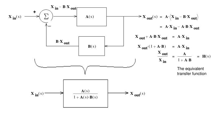
This is called a "closed loop" system, whereas a a system without feedback is called "open loop". The term "open loop" is often used to describe a system that is out of control.
