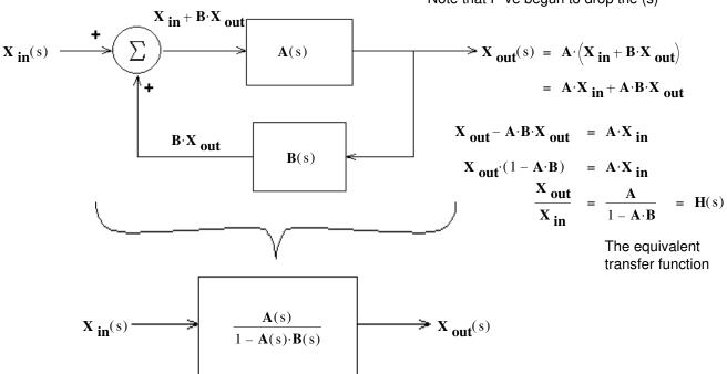
$\mathbf{A}(s) \cdot \mathbf{B}(s)$  is called the "loop gain" or "open loop gain"
