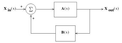
The entire loop can be replaced by a single equivalent block:
