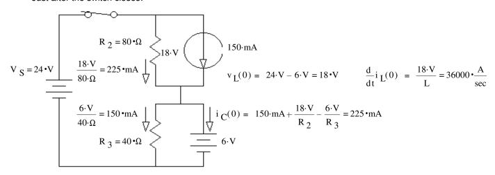
c) Find the initial condition and intial slope of  $v_C$  so that you could find all the constants in  $v_C(t)$ . Don't find  $v_C(t)$  or it's constants, just the initial conditions.
