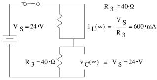
b) Find the initial condition and intial slope of  $i_L$  so that you could find all the constants in  $i_L(t)$ . Don't find  $i_L(t)$  or it's constants, just the initial conditions.
