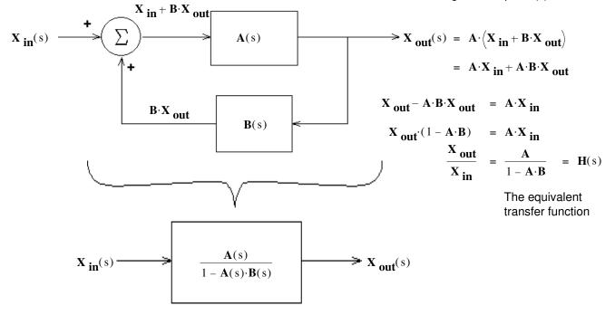
$A(s) \cdot B(s)$  is called the "loop gain" or "open loop gain"
