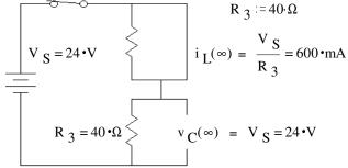
b) Find the initial condition and initial slope of  $i_L$  so that you could find all the constants in  $i_L(t)$ . Don't find  $i_{I}(t)$  or it's constants, just the initial conditions.
