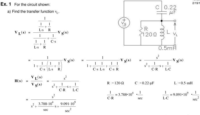
b) Find the characteristic equation for this circuit.
