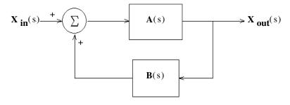
The entire loop can be replaced by a single equivalent block:
