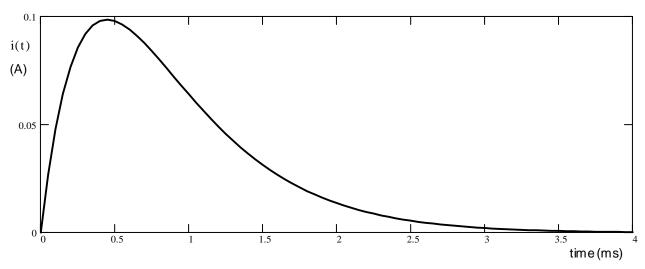
if you notice a remarkable similarity with the overdamped case, that's common for critical damping.
