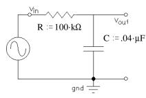
$$\frac{\mathbf{V}_{out}}{\mathbf{V}_{in}} = \frac{\frac{1}{j \cdot \omega \cdot C}}{\frac{1}{j \cdot \omega \cdot C} + R} = \frac{1}{1 + R \cdot (j \cdot \omega \cdot C)} = \mathbf{H}(\omega) = \text{The "Transfer Function"}$$
