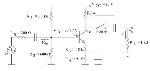
a) When the switch is open, the peak-to-peak output signal voltage at the collector is 4 Vpp. When the switch is closed this voltage drops to 2.88 Vpp. What is the output resistance of this amplifier?
