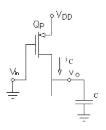
$$t_{PLH} = \frac{2 \cdot C}{k'_{p} \cdot \frac{W_{p}}{L_{p}} \cdot \left(V_{DD} - \left|V_{tp}\right|\right)} \cdot \left(\frac{\left|V_{tp}\right|}{V_{DD} - \left|V_{tp}\right|} + \frac{1}{2} \cdot ln \left(\frac{3 \cdot V_{DD} - 4 \cdot \left|V_{tp}\right|}{V_{DD}}\right)$$
