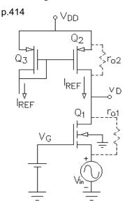
Source is the signal input, so let's assume the body is hooked to ground. Gate is at signal ground, so..
