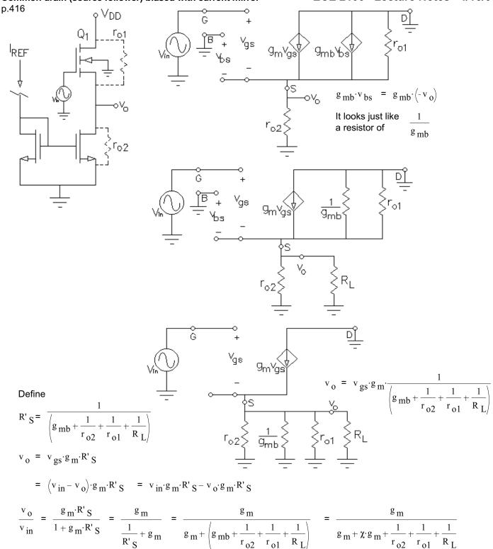
To find  $R_o$ , zero  $v_{in}$ , then you'll notice that  $v_{gs} = v_{bs}$ , so by the same type of analysis used on  $g_{mb}$ ,  $1/g_m$  just looks like another resistor in parallel with  $1/g_{mb}$ .
