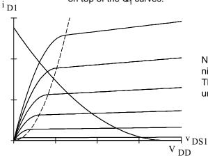
Notice that the new "load line" curves up. Its non-linearity will nicely offset the inherent  $i_D$  vs  $v_{GS}$  non-linearity of the  $Q_1$ . This results in a very linear transfer characteristic and an unexpected sq root in the gain term. Too bad the gain stinks.
