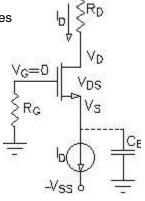
Note this particular arrangement doesn't have voltage gain unless the current source is bypassed, a rare thing in ICs since capacitors are so expensive to make in silicon.
