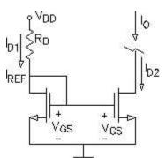
$$I_{D2} = \frac{1}{2} \cdot k'_{n} \cdot \frac{W_{2}}{L_{2}} \cdot (V_{GS} - V_{t})^{2}$$
