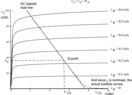
Similar analysis can be used with diode curves (see p157 & p273 in your textbook. Load lines can be helpful in visualizing the output limits and the optimal Q-point, but that's about all.
