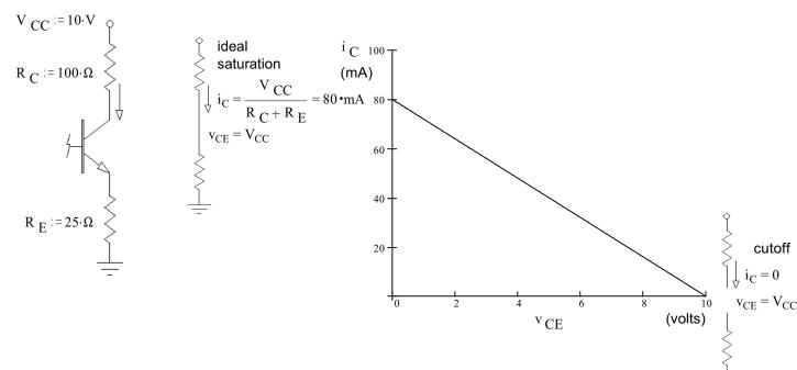
The load line is typically drawn right on top of the transistor's characteristic curves
