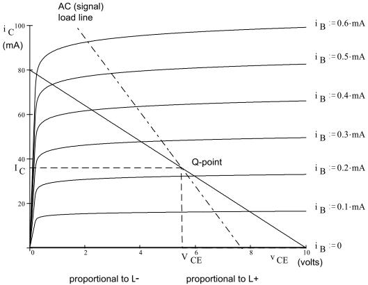
Actually, the slope of the AC (signal) load line is  $-\frac{1}{r_c + r_e + R_e}$
