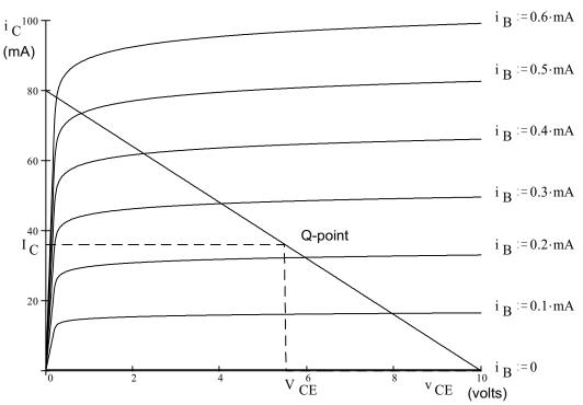
The slope of the load line is  $-\frac{1}{R_C + R_B}$
