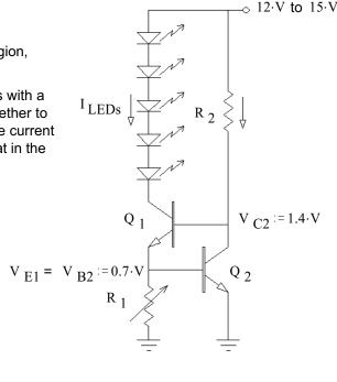
When enough current flows through R to get 0.7V across it, then the transistor will start to turn on to supply more current to the load. You could put a diode in the ground connection of the regulator to make up for the lost 0.7V across R.
