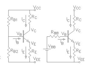
If you can neglect the base current,  $I_B$ . In that case:  $V_B = V_{BB}$   $V_E = V_{B^{-0.7} \cdot V}$   $I_E = \frac{V_E - V_{EE}}{R_E} I_C$
