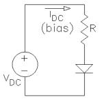
The result would be a bias current through the diode and a bias voltage across the diode.
