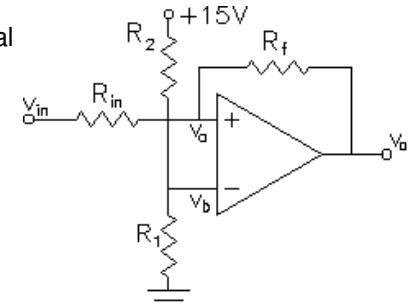
$$V_{sw2} = v_b + \frac{R_{in}}{R_f} \cdot (v_b - v_{o2})$$
