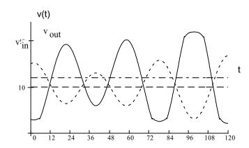
The signal is considered the AC (changing) part of the waveform and the DC is called "bias" or the "quiescent - point" (Q - point) of the circuit.
