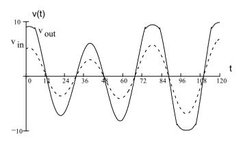
Many of the transistor amplifier circuits that we'll see this semester will have DC offsets and will invert the signal.
