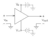
Batteries or power supplies are rarely shown on the schematic.
