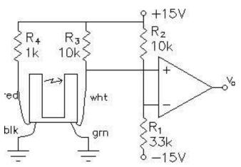
"interrupted" and when it is not. That's why you'd use a comparator in this situation— to provide a positive switching action at some level of beam interruption. (Some interrupters have comparators built in.) Observe the comparator output with the scope as you move the test slide. Comment in your notebook.
