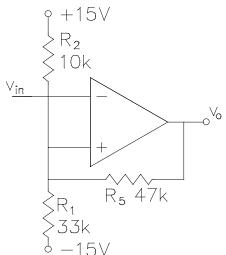
(4 pts) Hook the interrupter back to the input and play with the fuzzy side of the slide again. Move the slide back and forth where the switching occurs. You'll find that it always takes a significant movement to make the output switch. Comment in your notebook. Does this circuit have better noise immunity?
