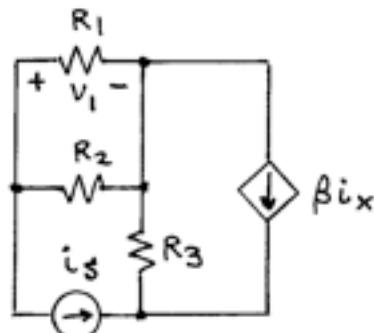
Careful inspection reveals that  $R_1$  and  $R_2$  are in parallel and  $i_s$  flows thru  $R_1$  and  $R_2$ .
