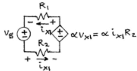
$$V\text{-loop: } V_S + i_{x1}R_1 - i_{x1}\alpha R_2 + i_{x1}R_2 = 0 \text{ V}$$
