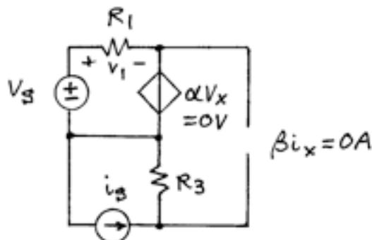
From the v-loop in the upper left we have  $v_1 = V_S$ .
