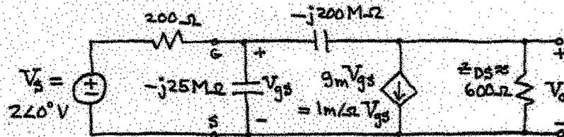
We now analyze the dependent source so we can replace it with an impedance,  $z_{eg}$ .
