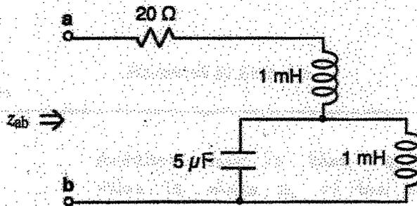
Find a frequency,  $\omega$ , that causes  $z_{ab}$  to be real, (i.e., imaginary part equals zero).
