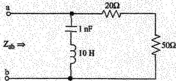
Find a frequency,  $\omega$ , that causes  $Z_{ab}$  to be real (i.e. imaginary part equals zero).
