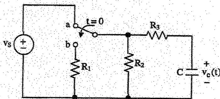
After being at position a for a long time, the switch moves to position b at time  $t = 0$ .
