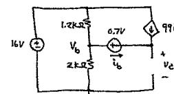
If we sum currents at node above C, we have  $-i_b - 99i_b = 0A \Rightarrow i_b = 0$ .
