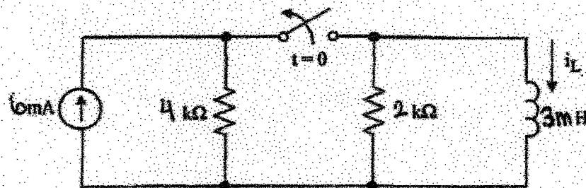
After being closed for a long time, the switch opens at  $t = 0$ . Find  $i_L(t)$  for  $t > 0$ .
