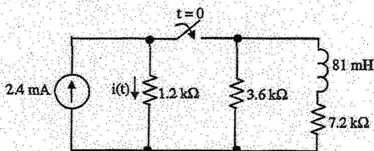
After being open for a long time, the switch is closed at  $t = 0$ .
