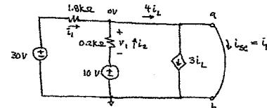
This is the same circuit as for  $t \rightarrow \infty$ . Using the value of 0V on the top node, we can find  $i_1$  and  $i_2$ :
