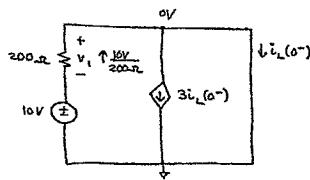
Because L = wire, we have 10V across  $200\Omega$  (so 10V src +  $v_{200\Omega} = 0 \text{ V}$ ).
