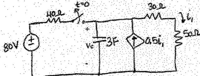
After being closed for a long time, the switch opens at  $t=0$ . Find  $V_c(t)$  for  $t > 0$ .
