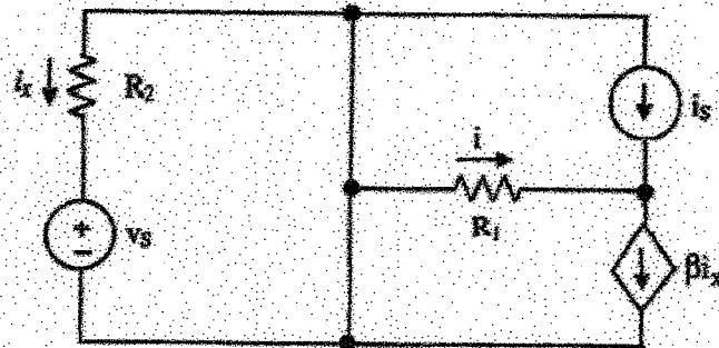
Using superposition, derive an expression for  $i$  that contains no circuit quantities other than  $i_s$ ,  $V_s$ ,  $R_1$ ,  $R_2$ , and  $\beta$ .
