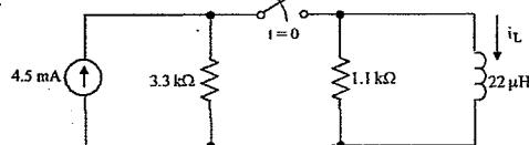
After being closed for a long time, the switch opens at  $t = 0$ . Find  $i_L(t)$  for  $t > 0$ .
