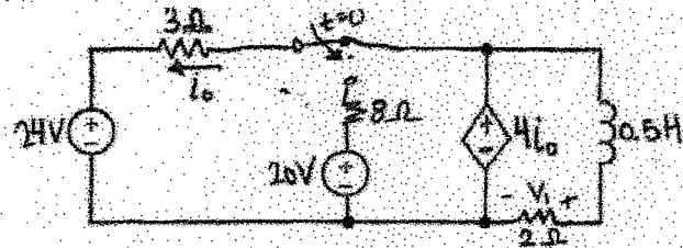
After being in the above position for a long time, the switch changes at  $t=0$ . Find  $v_L(t)$  for  $t > 0$ .
