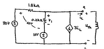
$$V_{Th} = V_{ab} \text{ open circ}$$
