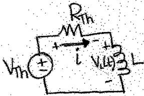
$$\begin{aligned} \text{V-loop} \\ +V_m - iR_m - V_c(t) = 0 \\ V_m - iR_m - L \frac{di(t)}{dt} = 0 \\ L \frac{di(t)}{dt} = +V_m - iR_m \end{aligned}$$
