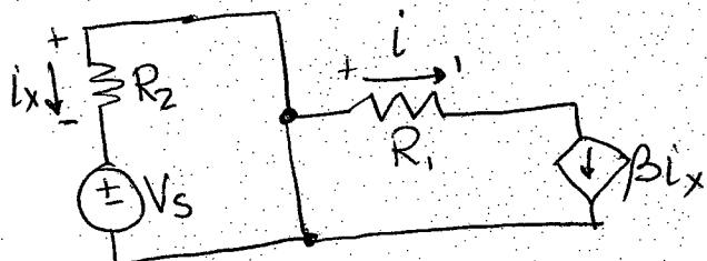
$$V\text{-loop: } +V_s + i_x R_2 = 0$$
