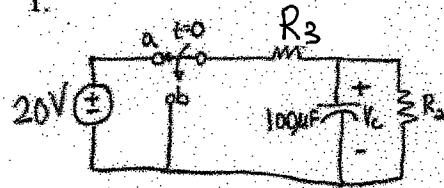
After being in position a for a long time, the switch moves to position b at  $t=0$ . Find  $R_2$  and  $R_3$  that gives the plot below for  $V_c(t)$ .
