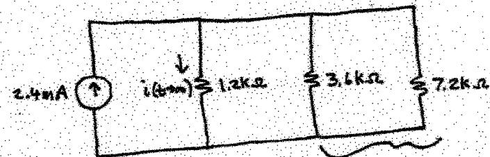
$$\begin{aligned} 3.6k\parallel 7.2k\Omega &= 3.6k\Omega \parallel 2 \\ &= 3.6k\Omega \cdot \frac{2}{3} \\ &= 2.4k\Omega \end{aligned}$$
