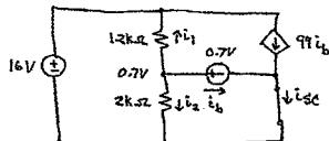
From current summation at node above  $C$ ,  $i_{sc} = i_b + 99i_b = 100i_b$ .
