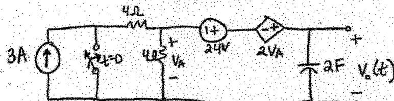
After being open for a long time, the switch closes at  $t=0$ . Find  $V_o(t)$  for  $t > 0$ .
