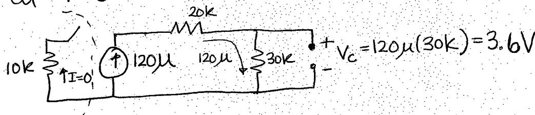
at  $t=0^+$ : (redraw circuit - voltage on cap cannot change instantaneously: use  $V_{source}$ )
