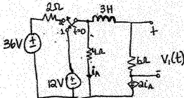
After being at position 1 for a long time, the switch moves to position 2 at  $t=0$ . Find  $v_1(t)$  for  $t > 0$ .
