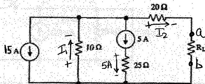
Calculate the value of  $R_L$  that would absorb maximum power, and calculate that value of maximum power  $R_L$  could absorb.
