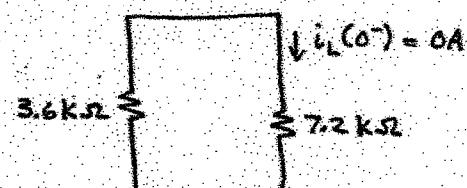
$t=0^+$ : L acts like current src of value  $i_L(0^+) = i_L(0^-) = 0A = \text{open circuit}$
