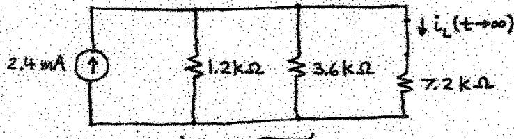
$$R_{\text{eq}} = 1.2 \text{ k}\Omega \parallel 3.6 \text{ k}\Omega = 1.2 \text{ k}\Omega \cdot \frac{1}{1+3} = 1.2 \text{ k}\Omega \cdot \frac{3}{4}$$
