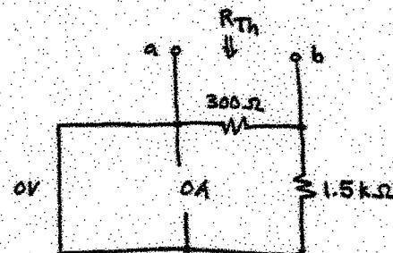
$$R_{Th} = 300\Omega \parallel 1.5k\Omega = 300\Omega \cdot 1 \parallel 5 = 300\Omega \cdot \frac{5}{6}$$
