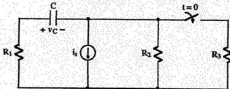
After being open for a long time, the switch closes at  $t = 0$ . Write an expression for  $v_C(t \geq 0)$  in terms of  $R_1$ ,  $R_2$ ,  $R_3$ ,  $i_s$ , and  $C$ .
