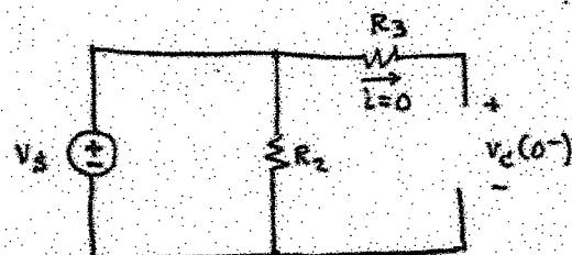
No current in  $R_3$  means no v-drop for  $R_3$ .
