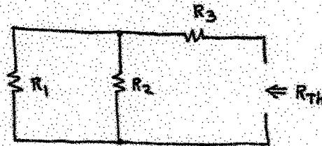
$$R_{Th} = (R_1 \parallel R_2) + R_3$$
