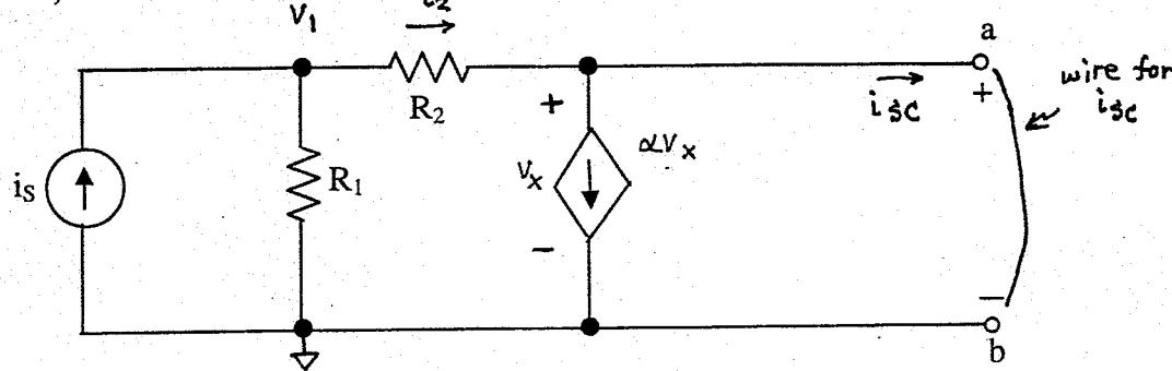
Find the Thevenin's equivalent circuit at terminals a-b.  $v_x$  must not appear in your solution. Hint: Use node voltage method to find  $v$  above  $R_1$ . Note:  $\alpha > 0$ .
