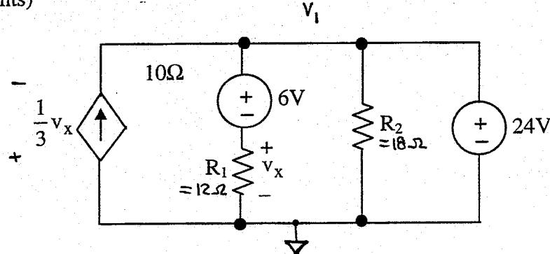
Calculate the power consumed by the dependent current source, (labeled  $\frac{1}{3}v_x$ ). Note: If a source supplies power, the power it consumes is negative.
