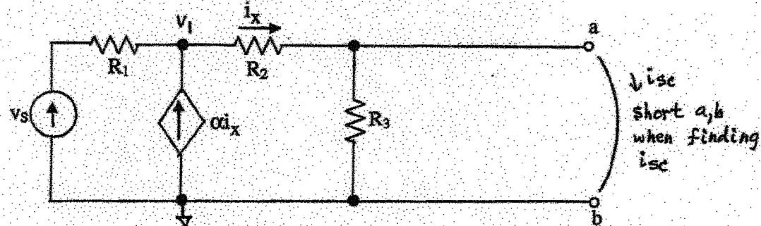
Find the Thevenin's equivalent circuit at terminals a-b.  $i_x$  must not appear in your solution. Hint: Use the node voltage method. Note:  $\alpha > 0$ .
