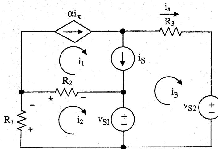
For the circuit shown, write three independent equations for the three mesh currents  $i_1$ ,  $i_2$ , and  $i_3$ . The quantity  $i_x$  must not appear in the equations.
