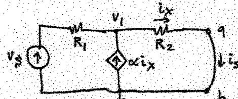
$$\text{Now, } i_{sc} = i_x = V_1 / R_2 = V_s / 1-\alpha$$
