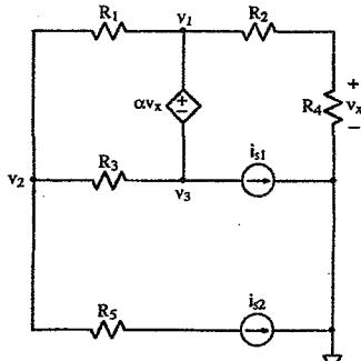
$$v_1 \left( \frac{1}{R_1} + \frac{1}{R_2 + R_4} \right) - v_2 \left( \frac{1}{R_3} + \frac{1}{R_1} \right) + v_3 \frac{1}{R_3} + i_{s1} = 0A$$
