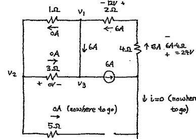
All the current will flow thru the wire between  $v_1$  and  $v_3$ , (path of least resistance).
