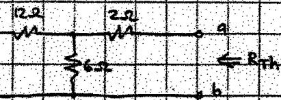
$$\begin{aligned} R_{TH} &= (4\Omega//12\Omega) + 2\Omega \\ &= 6\Omega \cdot \left( \frac{1}{2} \right) + 2\Omega \\ &= 6\Omega \cdot \frac{2}{3} + 2\Omega \\ &= 6\Omega \end{aligned}$$
