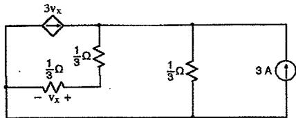
Calculate the power dissipated in the dependent current source, (labeled  $3v_x$ ).
