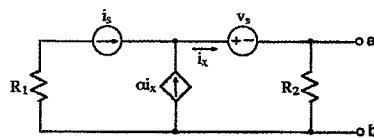
Find the Thevenin's equivalent circuit at terminals a-b.  $i_x$  must not appear in your solution. Note:  $\alpha \neq 1$ .
