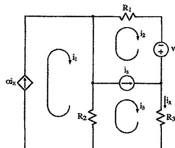
For the circuit shown, write three independent equations for the three mesh currents,  $i_1, i_2$ , and  $i_3$ . The quantity  $i_x$  must not appear in the equations.
