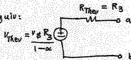
$$v_{\text{Thev}} = \frac{v_s R_3}{1-\alpha}$$
