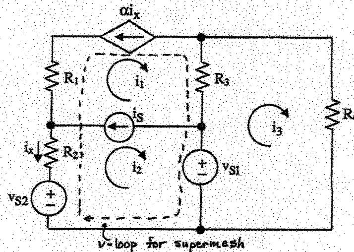
For the circuit shown, write three independent equations for the three mesh currents  $i_1$ ,  $i_2$ , and  $i_3$ . The quantity  $i_x$  must not appear in the equations.
