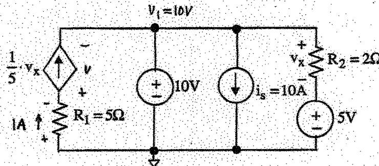
Calculate the power consumed by the dependent current source, (labeled  $\frac{1}{5}v_x$ ). Note: If a source supplies power, the power it consumes is negative.
