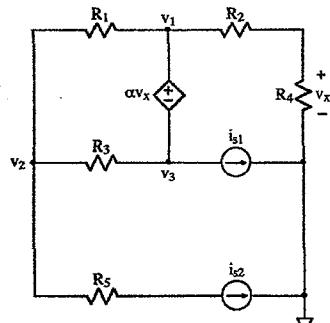
For the circuit shown, write three independent equations for the node-voltages,  $v_1$ ,  $v_2$ , and  $v_3$ . The quantity  $v_x$  must not appear in the equations.
