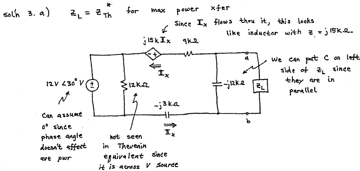
Circuit for determining Thvenin equivalent:
