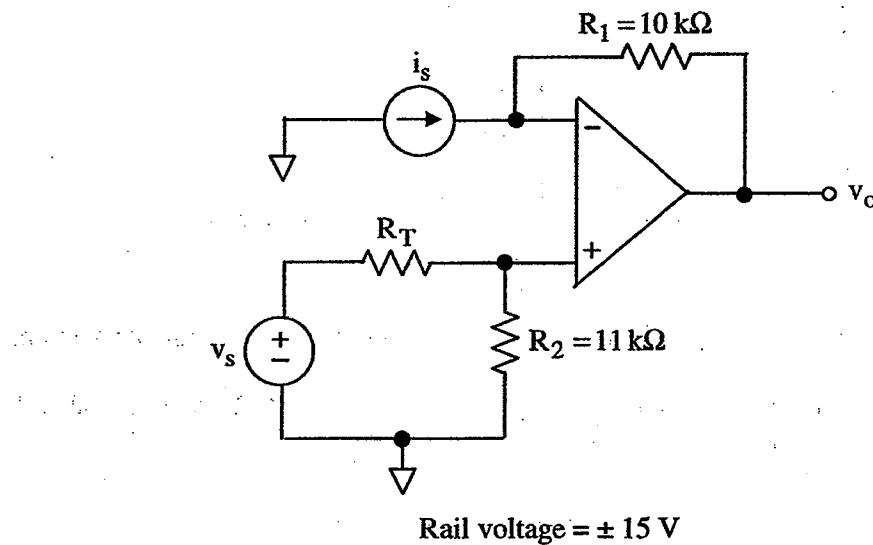
Design an electronic thermometer using the circuit diagram shown above. The voltage  $v_o$  is used to indicate temperature. Use a thermister with a resistance described by
