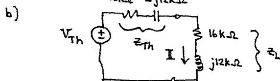
$$P \equiv (\text{ave pwr in } z_L) = \frac{|I|^2}{2} R \quad \text{where } R = 16k\Omega \text{ in } z_L$$
