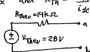
Sol'n: 3.b) Max pwr when  $R_L = R_{Ther} = 14\text{k}\Omega$
