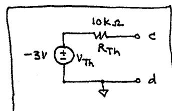
b)  $t > t_0$  switch is closed ( $-9V$  source and  $20k\Omega$  bypassed)
