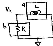
$$\begin{aligned} v_2(t > 0) &= v_2(t \rightarrow \infty) + [v_2(0^+) - v_2(t \rightarrow \infty)] e^{-t/\tau} \\ &= 0V + [v_2(0^+) - 0V] e^{-t/\tau} \\ &= v_2(0^+) e^{-t/\tau}, \text{ Now find } v_2(0^+). \end{aligned}$$
