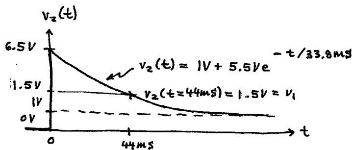
$$\text{Note: } R_{TH} C = \frac{22}{13} \text{ k}\Omega \cdot 20\mu\text{F} = 33.8 \text{ ms}$$
