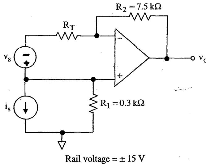
Design an electronic thermometer using the circuit diagram shown above. The voltage  $v_o$  is used to indicate temperature. Use a thermister with a resistance described by
