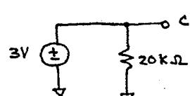
$$V_{Th} = 3V \text{ since } C \text{ connected to } 3V \text{ source}$$
