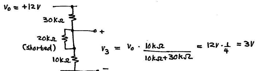
when  $v_o = -12V$ , top diode is forward biased = wire.
