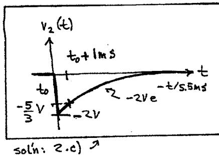
Let  $C = 1\mu\text{F}$ ,  $R = 5.5\text{k}\Omega$  or  $5.6\text{k}\Omega$  (standard value)
