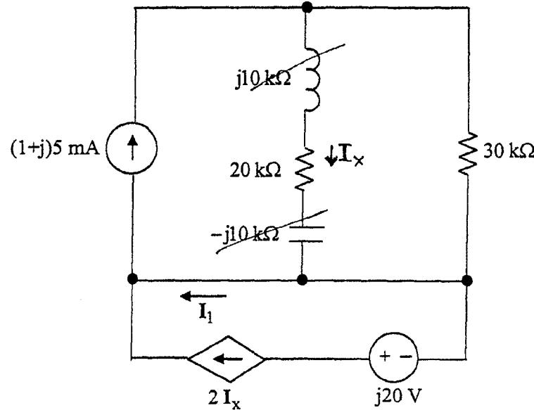
20 pts a. A frequency-domain circuit is shown above. Write the value of  $I_1$  in polar form.
