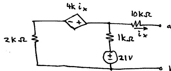
$$V_{Th} = V_{ab} \text{ open circuit}$$
