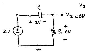
when switch closes,  $v_c$  will stay at 2V for  $t=t_0^+$ :
