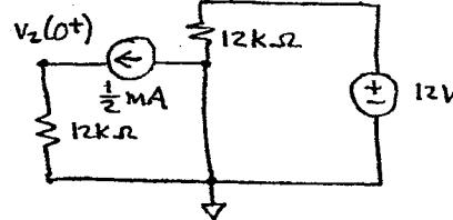
$$\begin{aligned} v_2(0^+) &= \frac{1}{2} mA \cdot 12k\Omega \\ v_2(0^+) &= 6V \end{aligned}$$
