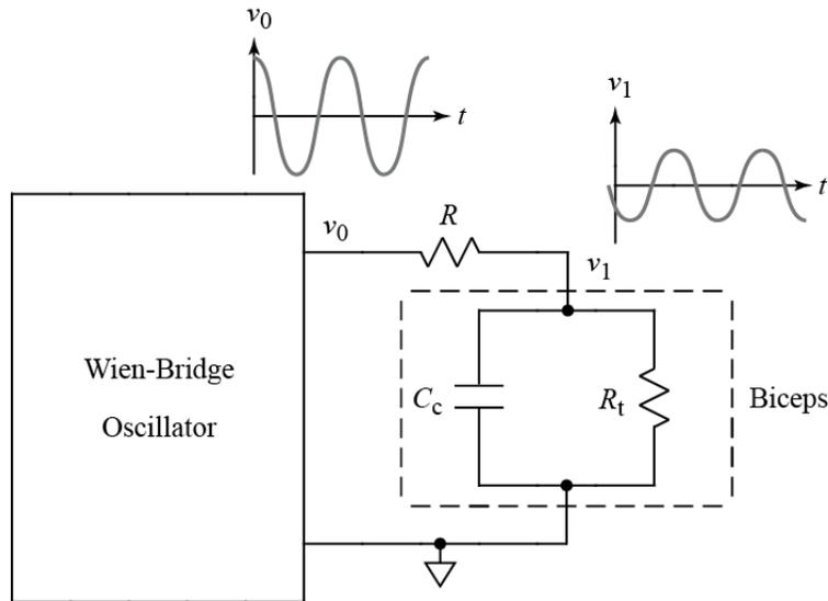
Figure 3. Block diagram of tissue measurement experiment.
