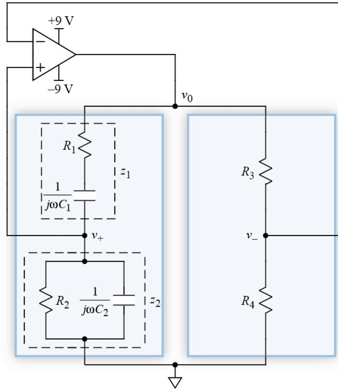
Figure 4. Wien-bridge oscillator schematic. Shaded boxes indicate voltage dividers.
