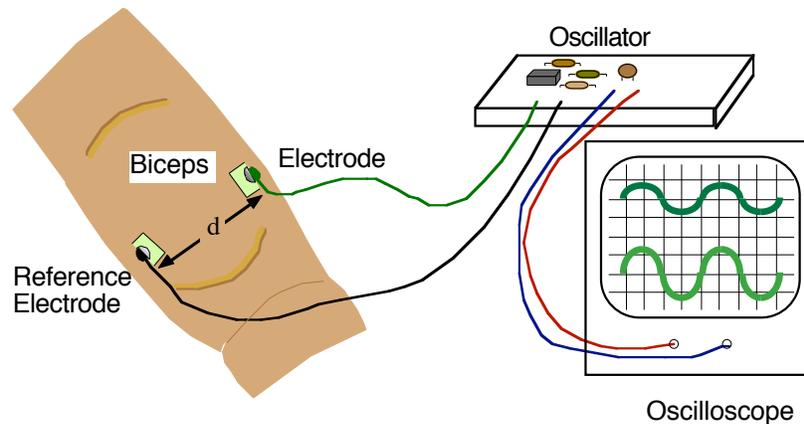
Figure 5. Tissue measurement configuration.
