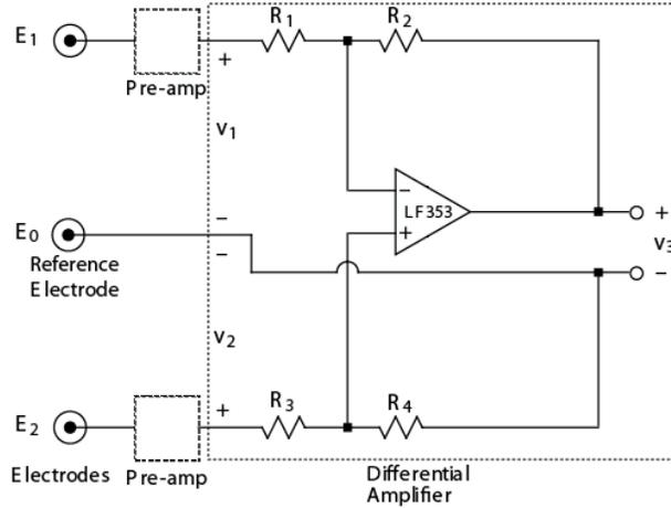
Figure 10. Schematic diagram of electromyogram circuit.
