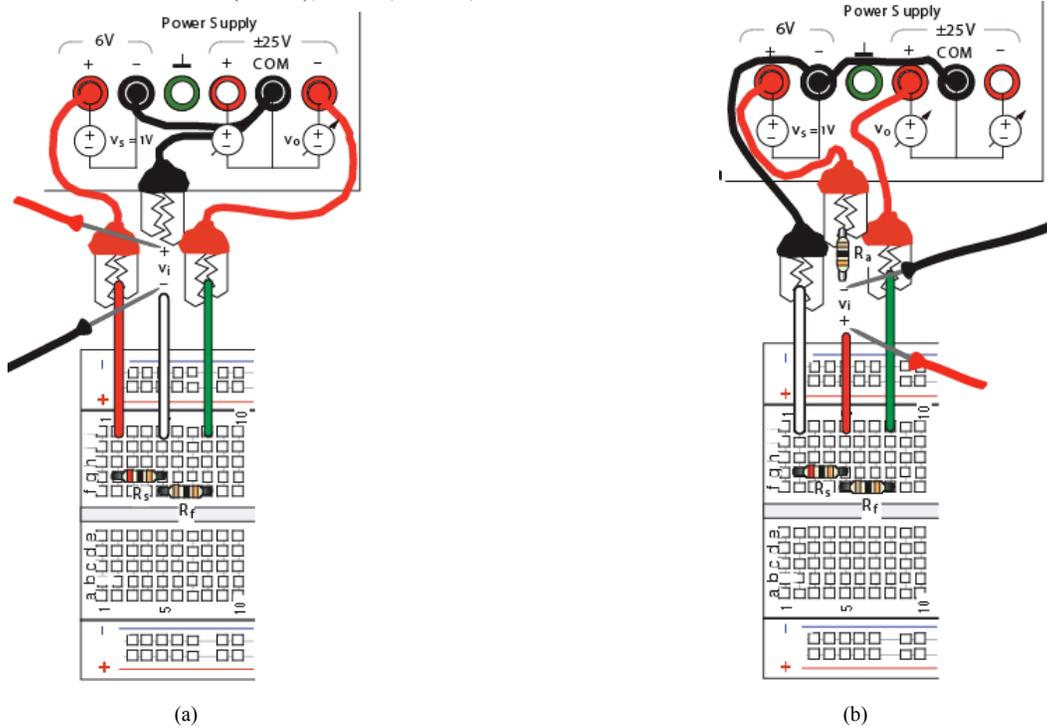
Figure 6. Protoboard layouts for modeling op-amp circuits and measuring  $v_i$ : (a) negative-gain op-amp circuit, (b) positive-gain op-amp circuit.
