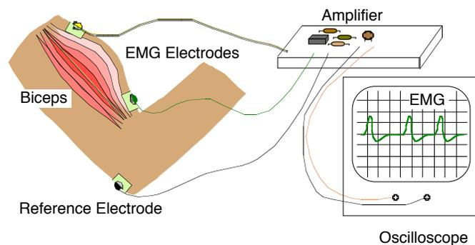
Figure 1. System for measuring an electromyogram.
