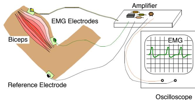
Figure 1. System for measuring an electromyogram.
