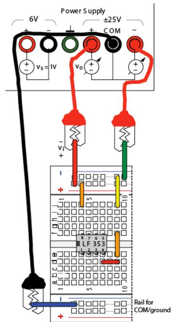
Figure 9. Protoboard and power-supply connections for power to op-amp.
