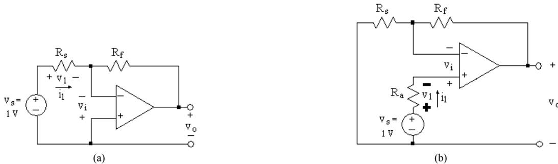
Figure 3. Simple op-amp circuits: (a) negative-gain circuit, (b) positive-gain circuit.
