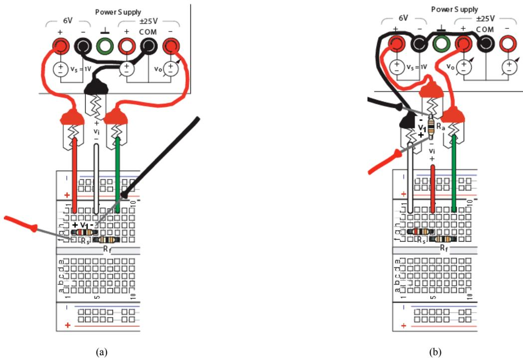
Figure 7. Circuits for modeling op-amp circuits and measuring  $v_1$ : (a) Negative-gain op-amp circuit, (b) Positive-gain op-amp circuit.
