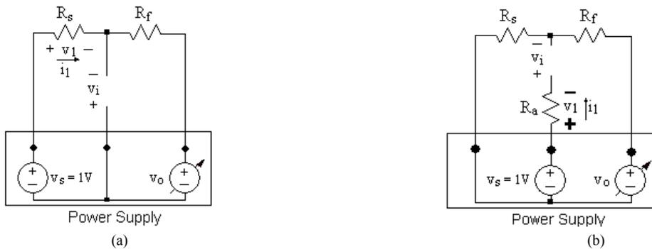
Figure 4. Circuits for modeling op-amp circuits: (a) negative-gain op-amp circuit, (b) positive-gain op-amp circuit.
