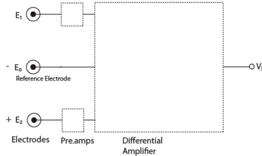
Figure 2. Block diagram of an electromyogram circuit.
