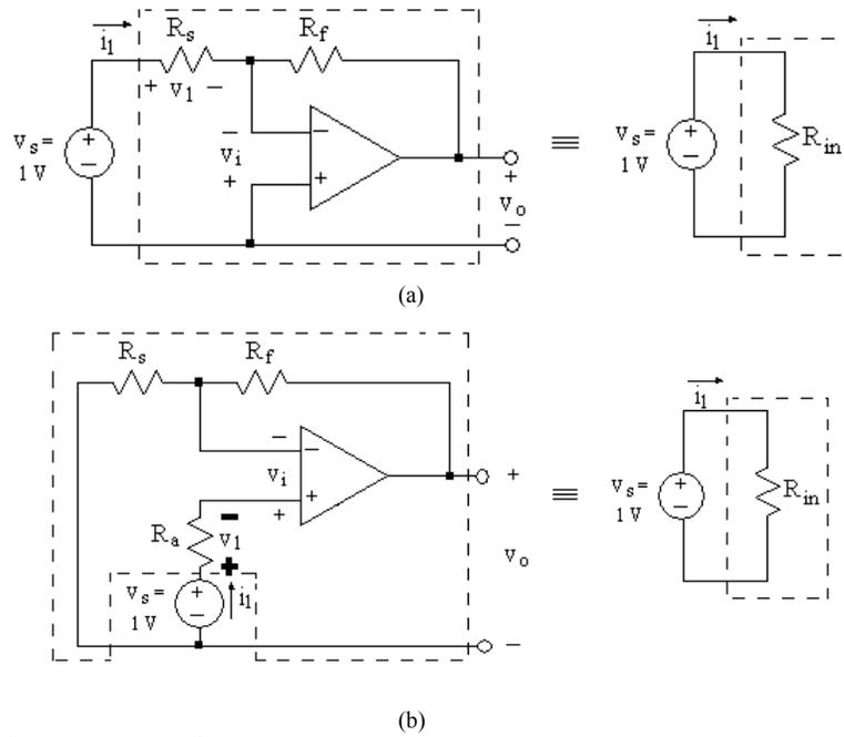
Figure 8. Input resistance  $R_{in}$  for pre-amp circuits: (a) negative-gain circuit (b) positive-gain circuit
