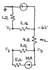
since no current. Flows in the 4.2 resistor, the voltage drop across it is zero. Thus, v3 = -6V. thru 452 resistor since there is no other path by which current can flow out to maintain a net zero charge, as required by Kirchhoff's (aw. (Consider a bubble around the bottom of the circuit. The current out of the babble must be zero.)
