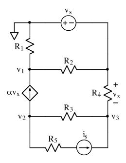
For the circuit shown, write three independent equations for the node-voltages,  $v_1$ ,  $v_2$ , and  $v_3$ . The quantity  $v_x$  must not appear in the equations.
