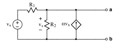
Find the Thevenin equivalent circuit at terminals a-b.  $v_x$  must not appear in your solution. **Hint:** use the node-voltage method.
