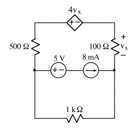
Calculate the power dissipated by the dependent voltage source, (labeled  $4v_x$ ).
