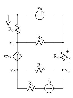
For the circuit shown, write three independent equations for the node-voltages,  $v_1, v_2$ , and  $v_3$ . The quantity  $v_x$  must not appear in the equations.
