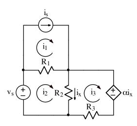
For the circuit shown, write three independent equations for the three mesh currents,  $i_1$ ,  $i_2$ , and  $i_3$ . The quantity  $i_x$  must not appear in the equations.
