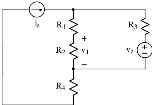
Derive an expression for  $v_1$ . The expression must not contain more than the circuit parameters  $v_a$ ,  $i_a$ ,  $R_1$ ,  $R_2$ , and  $R_3$ .
