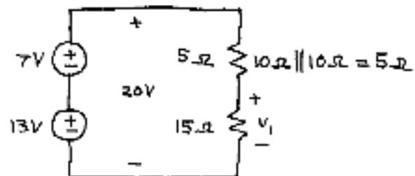
$$v_1 = 20V \cdot \frac{15\Omega}{5\Omega + 15\Omega} = 20V \cdot \frac{3}{4} \approx 15V$$
