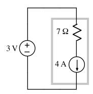
Find the total power dissipated by the components inside the box.
