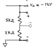
We have a voltage divider:  $v_3 = -12 \text{ V} \cdot \frac{5 \text{ k}\Omega}{2 \text{ k}\Omega + 5 \text{ k}\Omega} = -\frac{60}{7} \text{ V}.$
