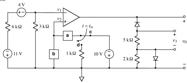
After being in position c for a long time, the switch moves from c to d at  $t = t_0$ .
