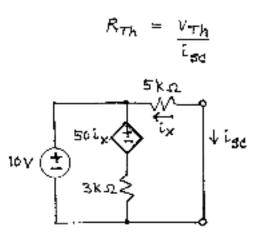
Although we have a dependent source, the IOV source between the top and bottom rails makes the 50ix and 3ks components irrelevant.
