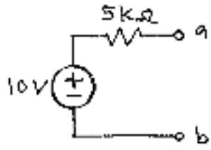
b)  $R_L = R_{Th} = 5\text{k}\Omega$  for max pwr transfer
