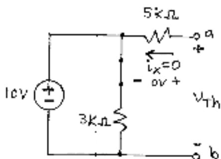
Since  $i_x = 0$ , there is no voltage drop across the  $5\text{k}\Omega$  resistor. An outer voltage loop reveals that  $V_{Th} = 10V$ .
