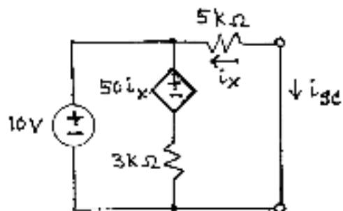
Although we have a dependent source, the 10V source between the top and bottom rails makes the  $50i_x$  and  $3k\Omega$  components irrelevant.
