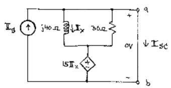
We observe that shorting a to be given over across the components in the middle. We suspect all of  $\mathbf{I}_S$  flows in the wire from a to b, meaning  $\mathbf{I}_{\mathbf{x}}=0$  and  $15\mathbf{I}_{\mathbf{x}}=0$  v.
