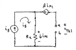
We observe that  $i_{Xl} = i_S$ , and  $v_{Thl} = i_{Xl}R_2 - \beta i_{Xl} = i_S(R_2 - \beta)$ (This is significantly simpler that the earlier superposition approach. There is more to be done before we are finished here, however.) case II: is off = open, vs on
