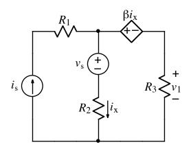
Using superposition, derive an expression for  $v_1$  that contains no circuit quantities other than  $i_s$ ,  $v_s$ ,  $R_1$ ,  $R_2$ ,  $R_3$ , and  $\beta$ , where  $\beta > 0$ .
