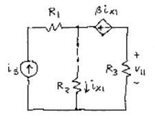
Note: Since R<sub>1</sub> is in series with a current source and the problem does not ask about ior & for R<sub>1</sub>, we may ignore R<sub>1</sub> and replace it with a wire.
