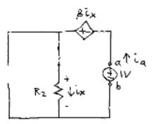
From v-loop on the right side, we have  $i_X R_Z - \beta i_X - IV = OV$ or  $i_X = \frac{IV}{R_Z - \beta}$ We also have that  $i_X = i_A$ .
