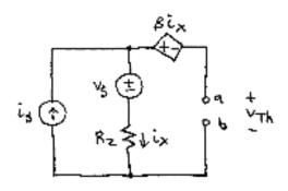
Now we use superposition or any other method of our choosing to find v<sub>th</sub>. As always, v<sub>th</sub> equals the open circuit voltage from a tob.
