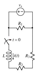
After being open for a long time, the switch closes at t = 0. Write an expression for  $i_L(t > 0)$  in terms of no circuit quantities other than  $R_1$ ,  $R_2$ ,  $R_3$ ,  $v_s$ , and L.
