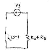
No current flows, owing to the open circuit.
