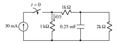
After being open for a long time, the switch closes at t = 0. Write a numerical expression for i(t) for t > 0.
