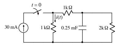
After being open for a long time, the switch closes at t = 0. Calculate the energy stored on the capacitor as  $t \rightarrow \infty$ .
