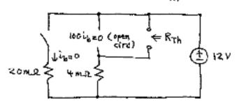
We observe that the Thevenin equivalent seen from the terminals where the L is connected is just the 4ms and 12V:
