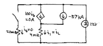
Because of the open circuit on the left, we have  $i_0 = 0$  and  $100i_0 = 0$ .
