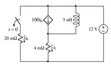
After being closed for a long time, the switch opens at t = 0. Find  $i_1(t)$  for t > 0.
