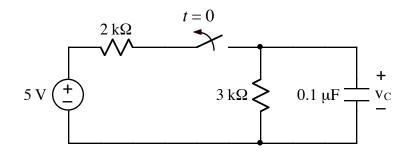
After being closed for a long time, the switch opens at t = 0. Find  $v_C(t)$  for t > 0. Hint: use a Thevenin equivalent for the voltage source and resistors for t < 0.
