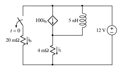
After being closed for a long time, the switch opens at t = 0. Find  $i_1(t)$  for t > 0.
