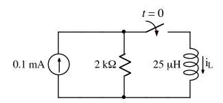
After being open for a long time, the switch closes at t = 0.  $i_L(t = 0^-) = 0$ A. Find  $i_L(t)$  for t > 0.
