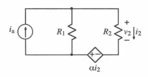
Derive an expression for  $v_2$ . The expression must not contain more than the circuit parameters  $\alpha$ ,  $i_a$ ,  $R_1$ , and  $R_2$ . Note:  $\alpha < 0$ .
