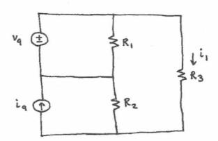
Derive expression for i. Expression must contain no other parameters than  $V_a$ , ia,  $R_1$ ,  $R_2$ ,  $R_3$ . sol'n: Use Kirchhoff's Laws. Label resistors.
