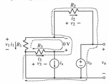
Looking first for components in series that carry the same current, we see that  $R_1$  and  $R_2$  have equal but opposite currents:
