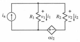
We look for components in series and find that only  $R_2$  and the dependent source are in series. This may prove useful later on, but gives us the current for a voltage source, which we may ignore when solving for  $v_2$ .
