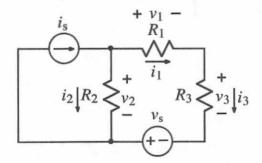
We observe that  $R_3$  is in series with  $R_1$  and carries the same current.
