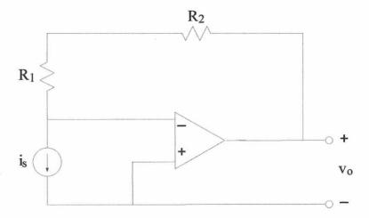
The op-amp operates in the linear mode. Using an appropriate model of the op-amp, derive an expression for  $v_0$  in terms of not more than  $v_s$ ,  $i_s$ ,  $R_1$ , and  $R_2$ .
