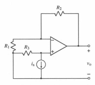
The op-amp operates in the linear mode. Using an appropriate model of the op-amp, derive an expression for  $v_0$  in terms of not more than  $i_s$ ,  $R_1$ ,  $R_2$ , and  $R_3$ .
