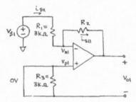
R3 is bypassed by a wire and may be ignored. The circuit is then seen to be a simple negative-gain amplifier:
