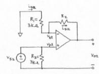
Since  $R_3$  is across V-source  $V_{\pm 2}$ , we may ignore it. The circuit is then seen to be a simple positive-gain amplifier:
