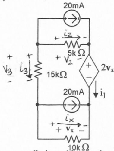
Find  $v_x$ ,  $i_1$ , and the power dissipated by the dependent source.
