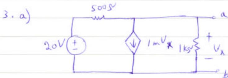
we can replace the dependant source with an equivalent resistance
