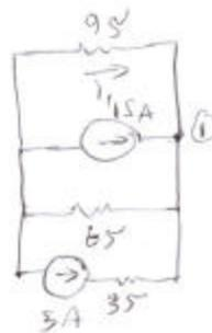
Since the two current sources contribute currents at the same direction to ~~node~~ node 1, and since we do not care about the voltage across the  $3\Omega$  resistor, we can again draw the circuit as follows.
