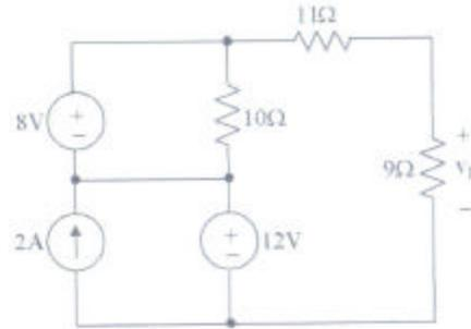
1) The voltage across the  $10\Omega$  resistor is equal to  $8V$  (parallel to the voltage source). We can redraw the right loop as follows
