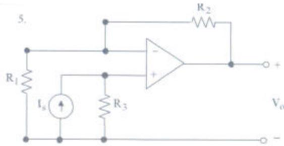
The op-amp operates in the linear mode. Using an appropriate model of the op-amp, derive an expression for  $V_o$  in terms of not more than  $I_s$ ,  $R_1$ ,  $R_2$ , and  $R_3$ .
