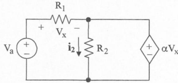
20 pts a) Drive the expression for  $i_2$  containing not more than circuit parameters  $\alpha$ ,  $R_1$ ,  $R_2$ , and  $V_a$ .
