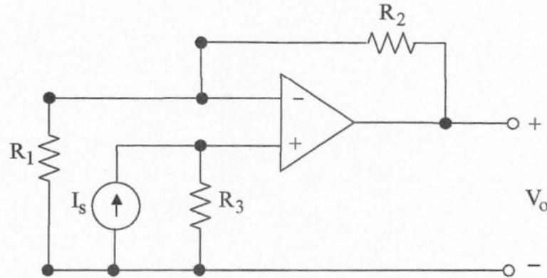
The op-amp operates in the linear mode. Using an appropriate model of the op-amp, derive an expression for  $V_o$  in terms of not more than  $I_s$ ,  $R_1$ ,  $R_2$ , and  $R_3$ .
