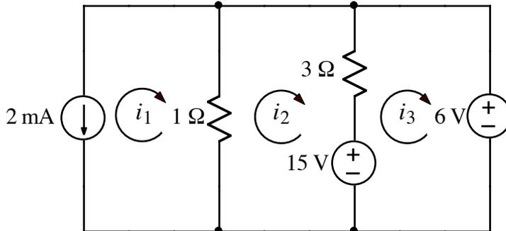
Use the mesh-current method to find  $i_1$ ,  $i_2$ , and  $i_3$ .
