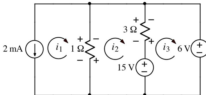
The current through the  $1\Omega$  resistor (measured with an arrow pointing down) is  $i_1 - i_2$ . The current through the  $3\Omega$  resistor (measured with an arrow pointing down) is  $i_2 - i_3$ .
