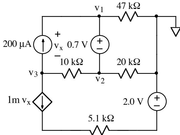
Use the node-voltage method to find  $v_1$ ,  $v_2$ , and  $v_3$ .
