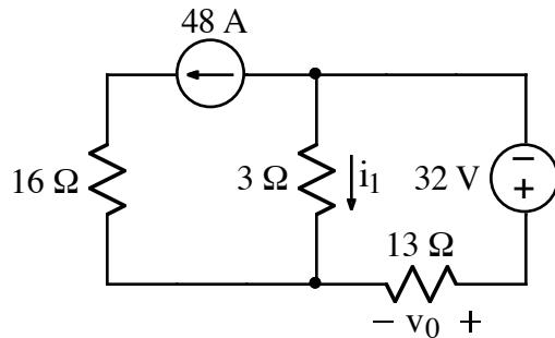
Use the node-voltage method to find  $i_1$  and  $v_0$ .
