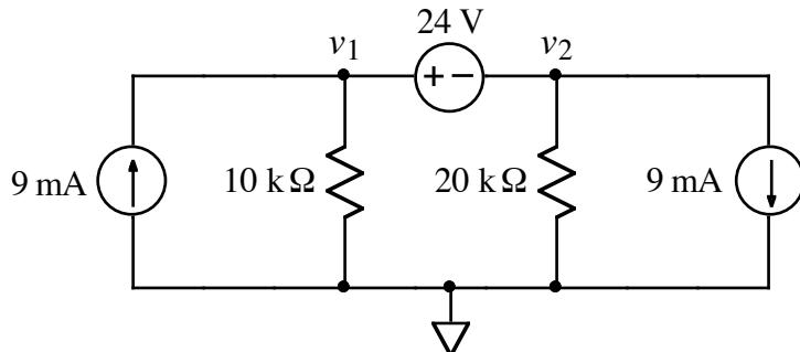
Use the node-voltage method to find  $v_1$  and  $v_2$ .
