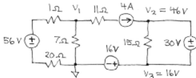
We find that  $V_2$  and  $V_3$  are known values, owing to the 16V and 30V sources connected in series to the reference node, (with no series resistors).
