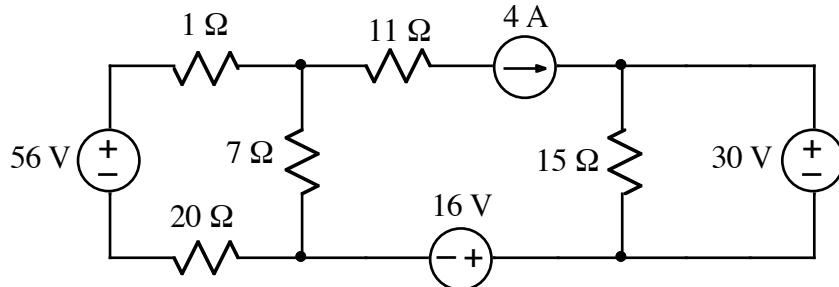
Choose a reference node and use the node-voltage method to the remaining node voltages.
